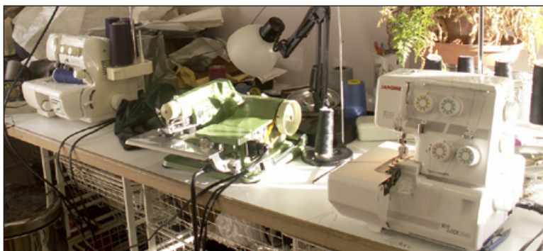
Specialty machines allow Ramona to perform high-quality work: at left is a cover-stitch machine for hemming and stitching on knits and fleece; center is a commercial blind-stitch machine for nearly-invisible hems; right is a serger that creates bound seams.
