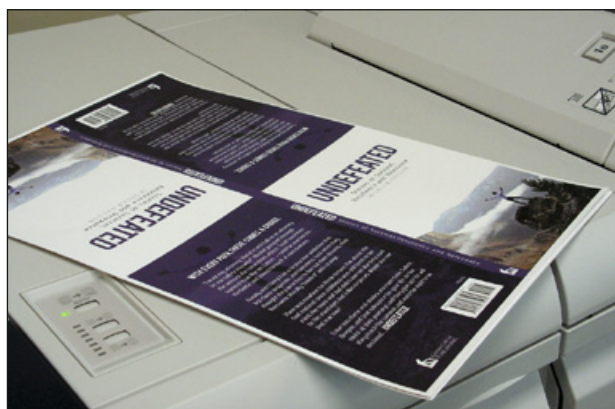
This book cover, printed on heavy stock, will be merged with the rest of the pages and output as a bound book with the optional finishing equipment provided with some machines.
